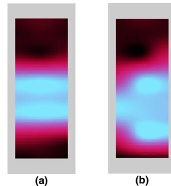
Fig. 2. BOS pressure images of subject during 2 stages of bed exit. (a) thighs are exerting uniform pressure while in sitting position (b) pressure shifts to torso and hands.
